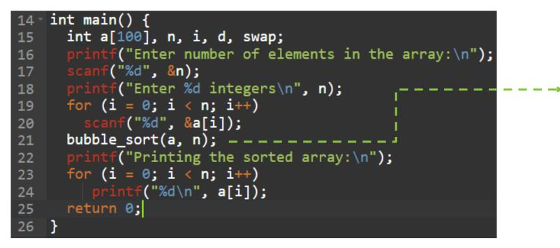
Values are passed to the function a = Array containing the elements/user input n= Total number of elements
