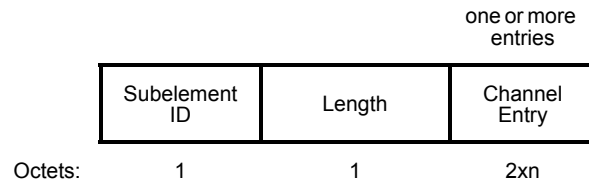
Figure 9-396—Location Indication Channels subelement
