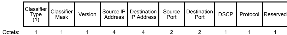
Figure 9-272—Frame Classifier field of Classifier Type 1 for traffic over IPv4
