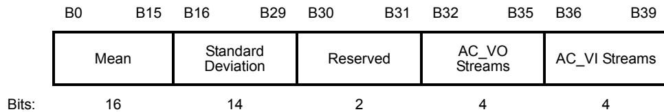
Figure 9-497—QLoad field format
