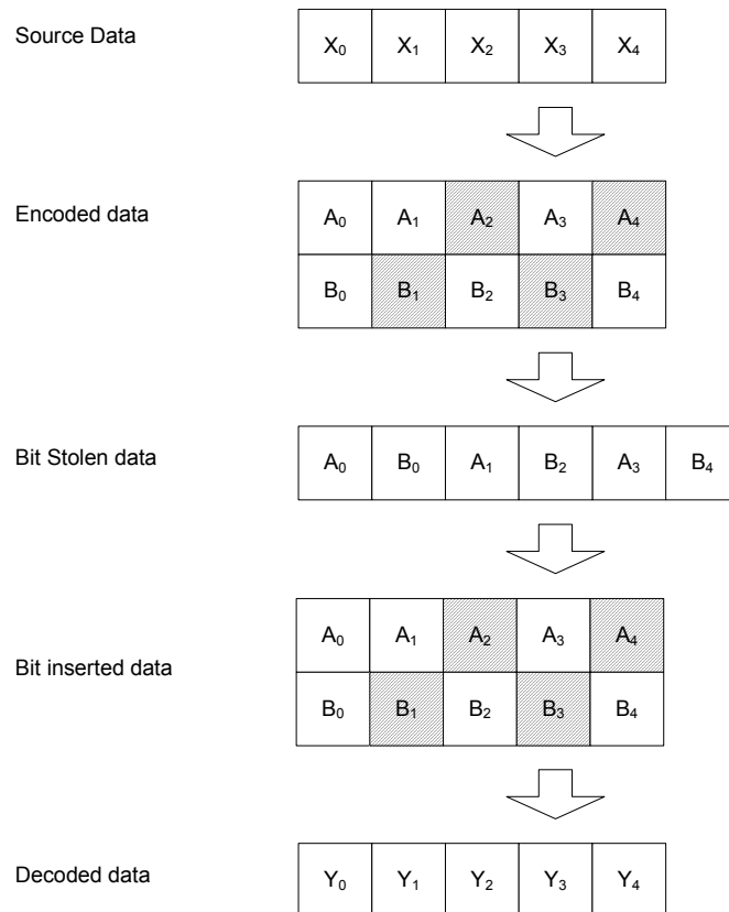
Figure 19-11—Puncturing at rate 5/6
