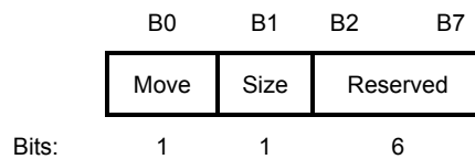
Figure 9-502—Change Type Bitmap field format
