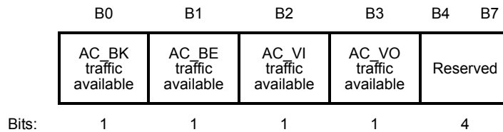
Figure 9-350—TPU Buffer Status Information field
